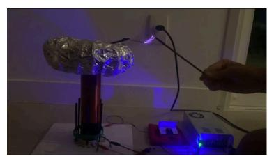
does not start as much, but, by timing the signal impulses from the primary coil, we can push the voltage in the secondary coil like a swing that keeps increasing its energy. This circuit, called the slayer exciter, does this automatically for us. Thus, the secondary coil quickly ramps up the voltage from 36 volts to 50 thousand volts in mere milliseconds.
